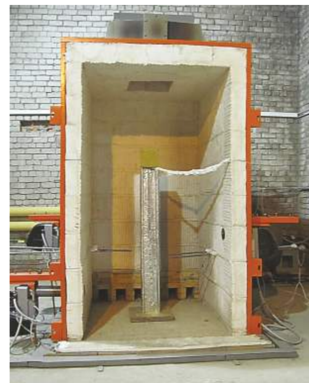
Universal furnace for fire tests of building structures
